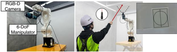
Figure 6. Hardware setup and the robot's field of view
