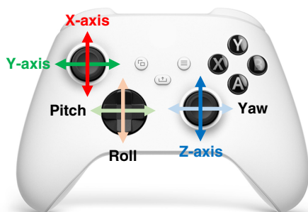
Fig. 11. Handheld controller (Xbox 360 controller) used in this study and its six-DoF mappings.
