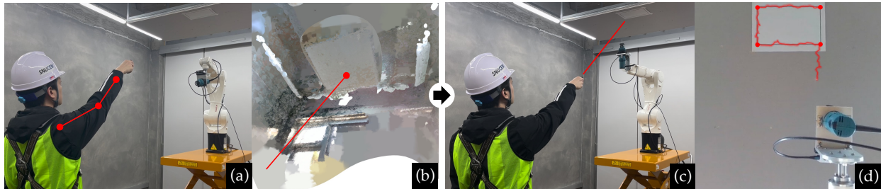
Figure 1. Task specification sequence using our gesture-based human-robot interface. (a-b): The human operator uses deictic gestures to indicate the target location; (c-d): After the robot moves to the detection pose, laser pointing is used to fine-tune the target location.
